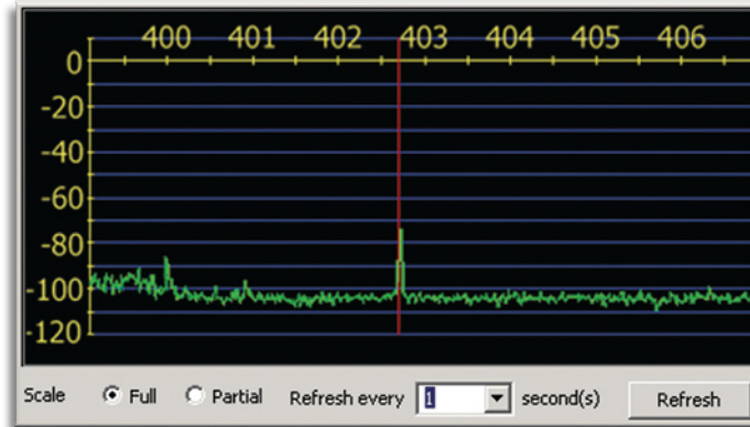
Finding a suitable frequency and monitoring telemetry is easy with a real-time spectrum display.
