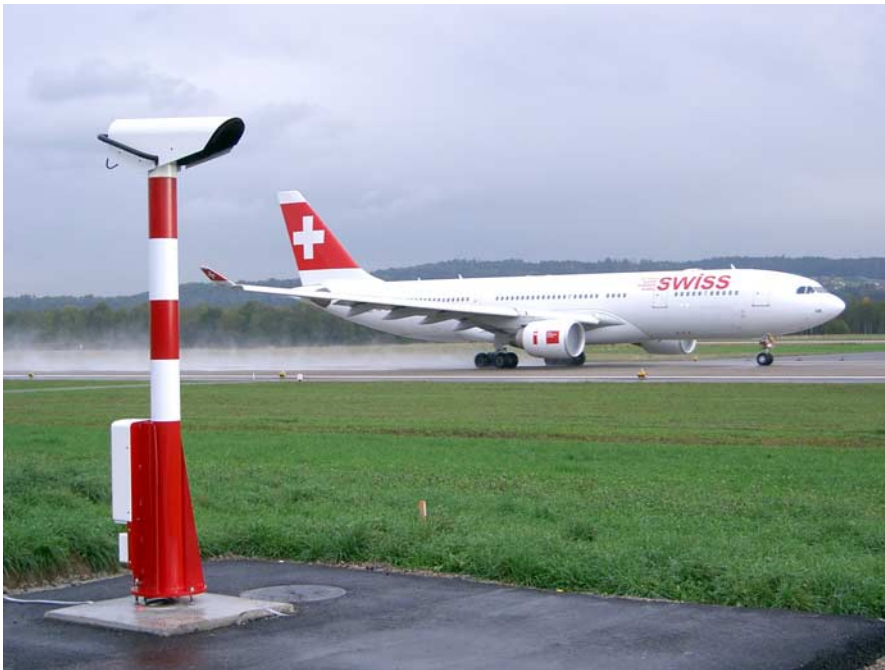
The Vaisala Transmissometer LT31 enables the accurate and reliable single baseline measurement for CATIIIb category airports.
